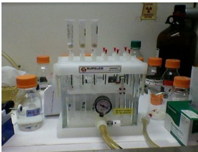
Figure B2. Cleaning and concentrating extracted chemicals with HLB cartridges with selected SPE methods
